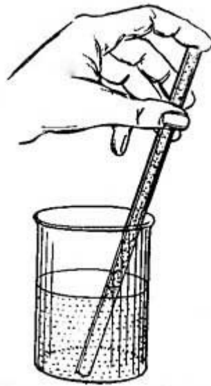
FIG. 3 —Water rises in the tube when the air is withdrawn.
