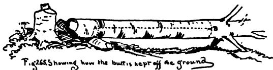
Fig. 265 Showing how the butt is kept off the ground
