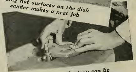
The edge of the tray can be molded on a shaper
